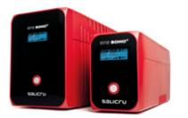
230v Input, 230v Output 50 or 60 Hertz Line interactive Topology Tower version Simulated Sinewave Inverter Transfer Time 2 to 6ms IEC Adapter Outputs Audible Alarms Internal Batteries only Cold Start
